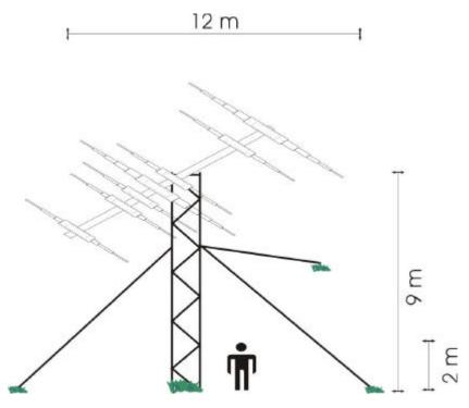
The picture shows a schematic drawing of the antenna installation. In real life, the tower is vertical and the antenna is horizontal. In other words, while the antenna appears slanted in the picture, it is in fact planar and can be easily avoided as a unit by a bird in flight. A human (size 2 m) is shown for perspective. The antenna's boom and elements are made from aluminium tubing and can be clearly seen at a distance.
